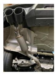
2. Next, you may install driver side muffler assy. #A onto the factory pipe using clamp #C.
