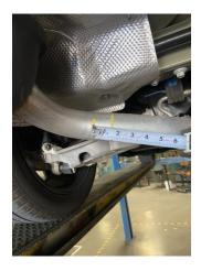
1. First you'll need to cut both tailpipes 1.5" from the beginning of each straight closest to the muffler, the cuts are marked in this photo. (BE SURE YOU CUT CORRECTLY). Once cut you may remove both muffler assembly's and clean the burr on both pipes that are still on the vehicle.
