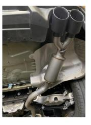
**3.** Now begin installing the passenger side muffler assy. **#B** using another clamp **#C**. Once finished you may install all tips **#D** onto the exits and tighten the exhaust.
